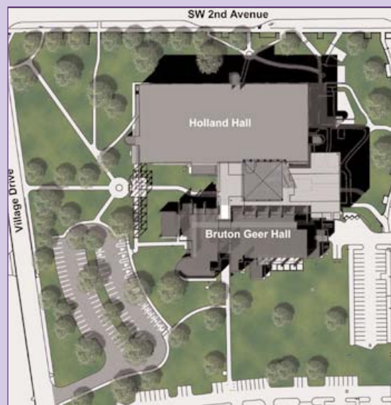
The first phase of construction will renovate/convert Holland Hall’s first two floors into library space and provide new classrooms on its third floor and as “infill” between Holland and Bruton-Geer Halls. The site west of both buildings will be developed as a plaza area and new staff parking.
